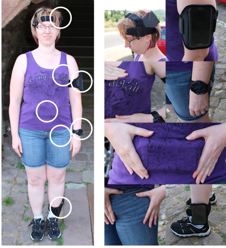
Fig. 1. Sensor placement. Each subject wore the wearable devices on the head, chest, upper arm, waist, forearm, thigh, and shin (top down).
