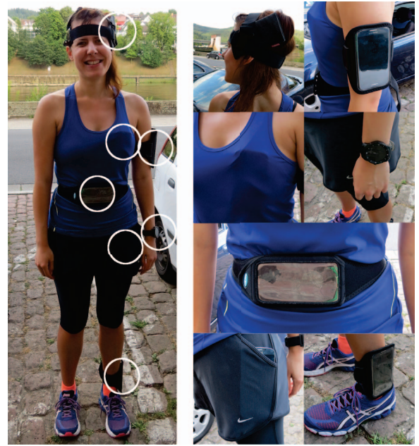
Fig. 1. Sensor placement. The subject wears the wearable devices on the head, chest, upper arm, waist, forearm, thigh, and shin (top down).
