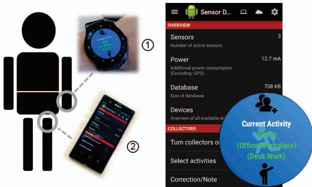
Fig. 2. Sensor Data Collector. The framework consists of a wear (1) and hand (2) app which allows to record each sensor that is available and provides labeling and visualization functions.
